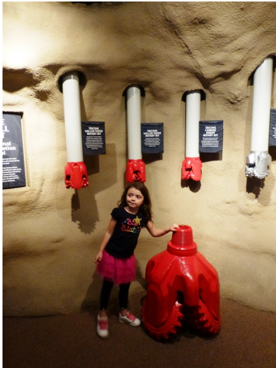
Drill bits used in the oil and gas industry. Exhibit at the Kern County Museum, Bakersfield Calif. A 5-year-old girl stands next to a 24-inch bit for scale.
