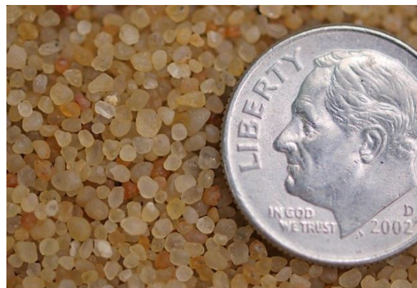
Fracking sand used as a proppant (Minnesota Environmental Board).
