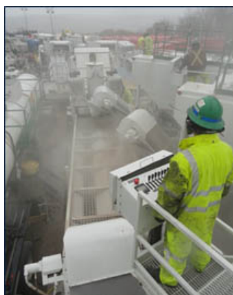
Silica dust surrounding worker conducting sand transfer operations. (NIOSH).
