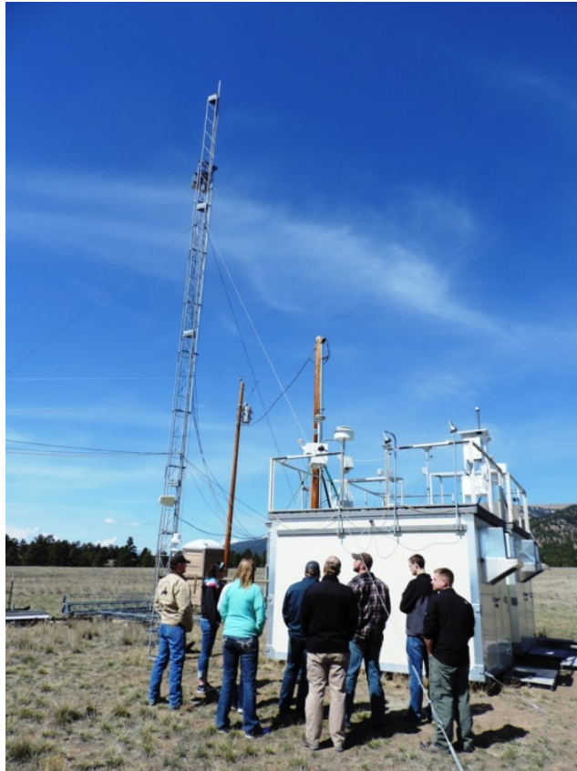
National ambient air monitoring station near Gates of the Mountain, Montana, where the six EPA primary pollutants are monitored.
