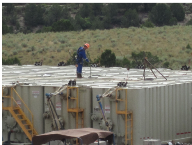
A flowback technician gauging a flowback tank through a hatch at the top of the tank. (CDC photo).
